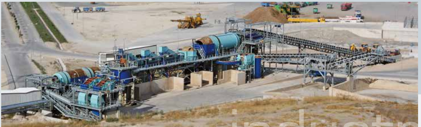
■ Beet Washing Plant: Drum beet washer (500 t/h)
